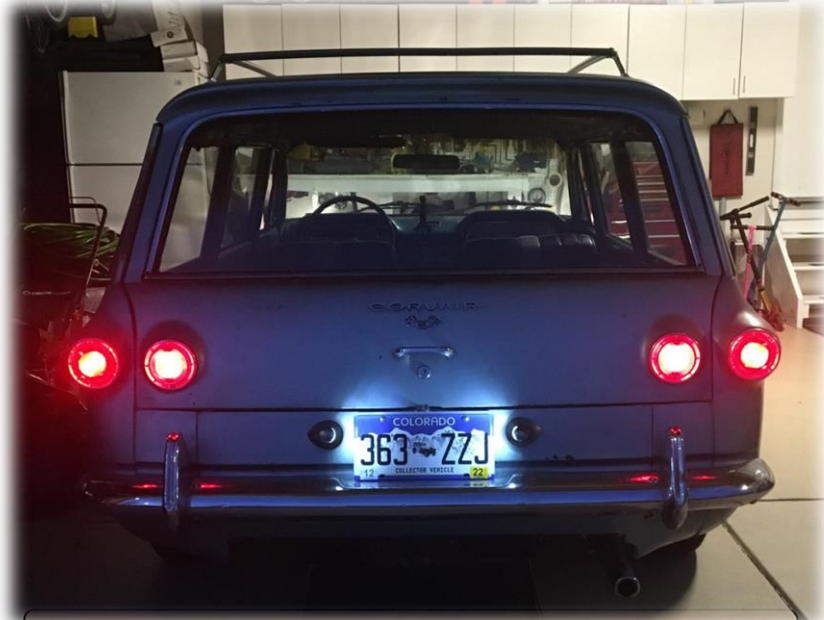
After-install of the red LED 1157 bulbs in the rear of the wagon.
