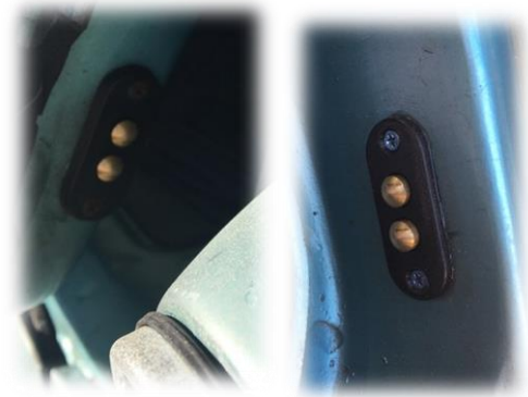
W.I.D.E. (wires in doors eliminated) solution for independent current to each
