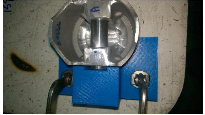
I also made up a stop for inserting the pins when installing the rods.
