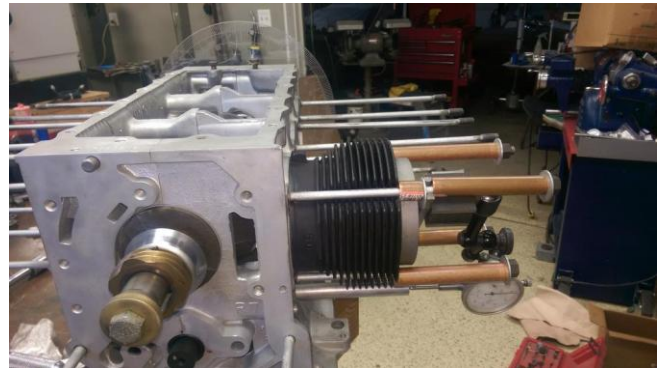
Here pressing on the cam gear.
