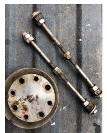
I keep four 1/4-20 bolts that are three inches long, [secured] nearby to my 'greaser', to ease the installation.
