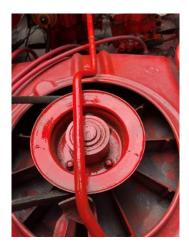
The four bolts that hold the Blower onto the Bearing can be removed without even loosening the belt.
