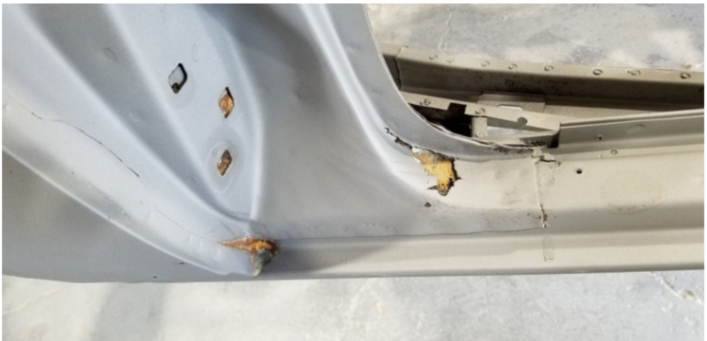
Driver's door sill corrosion, front. This area was previously covered with Bondo.
