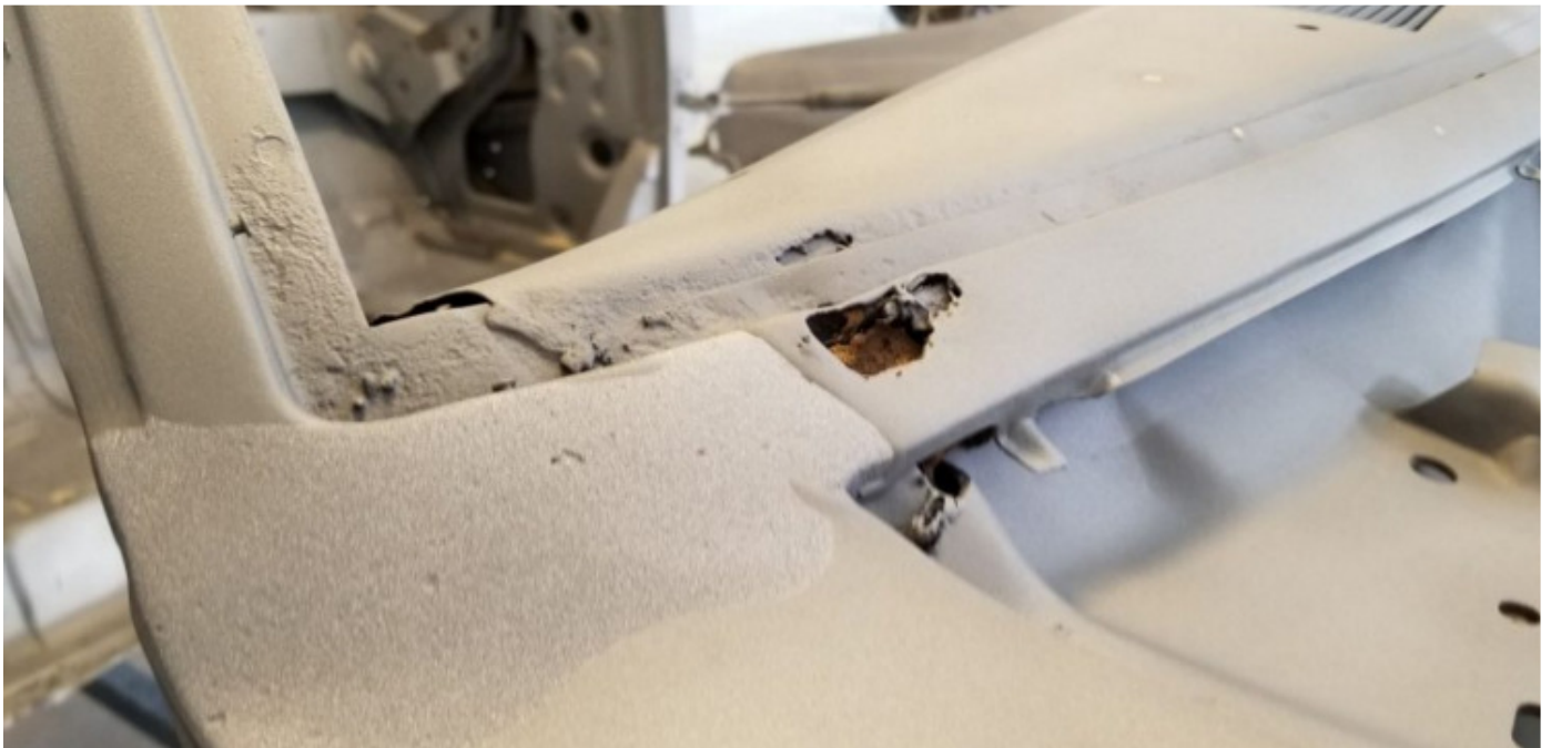
Cowl corrosion, beneath the windshield. This will be replaced with a full-width new piece
