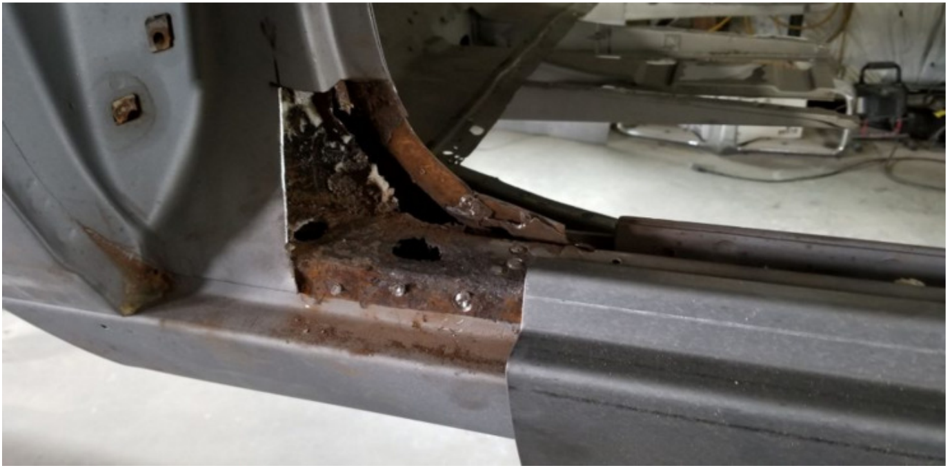
Same area, with the metal cut away for a patch panel.
