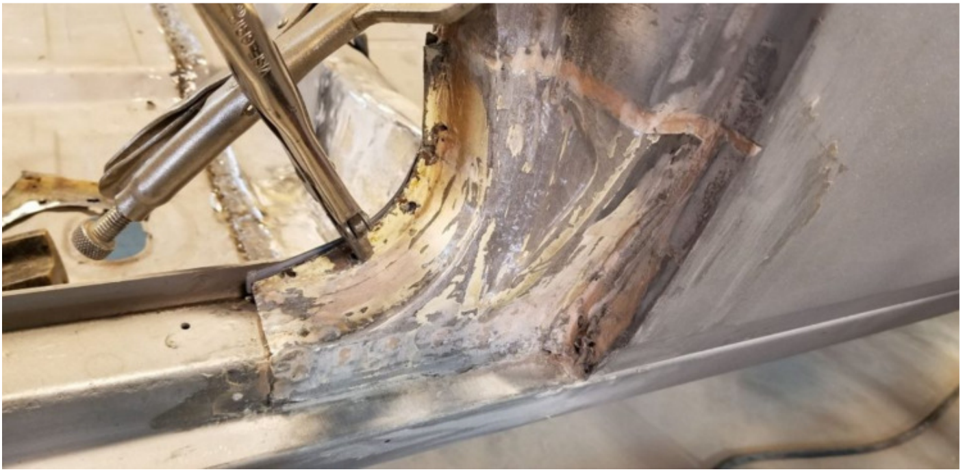
The repaired driver's door sill, rear.
