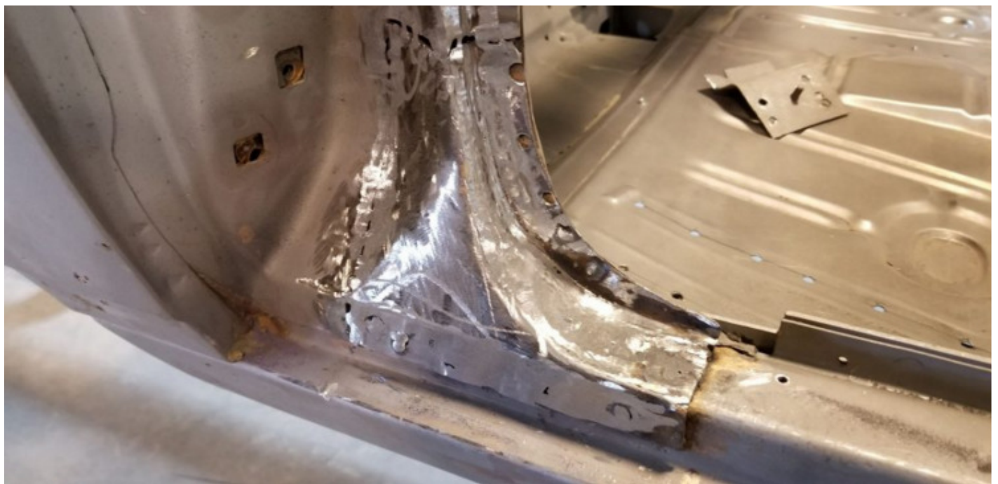
The front of the driver's door sill, with the patch panel welded in place.
