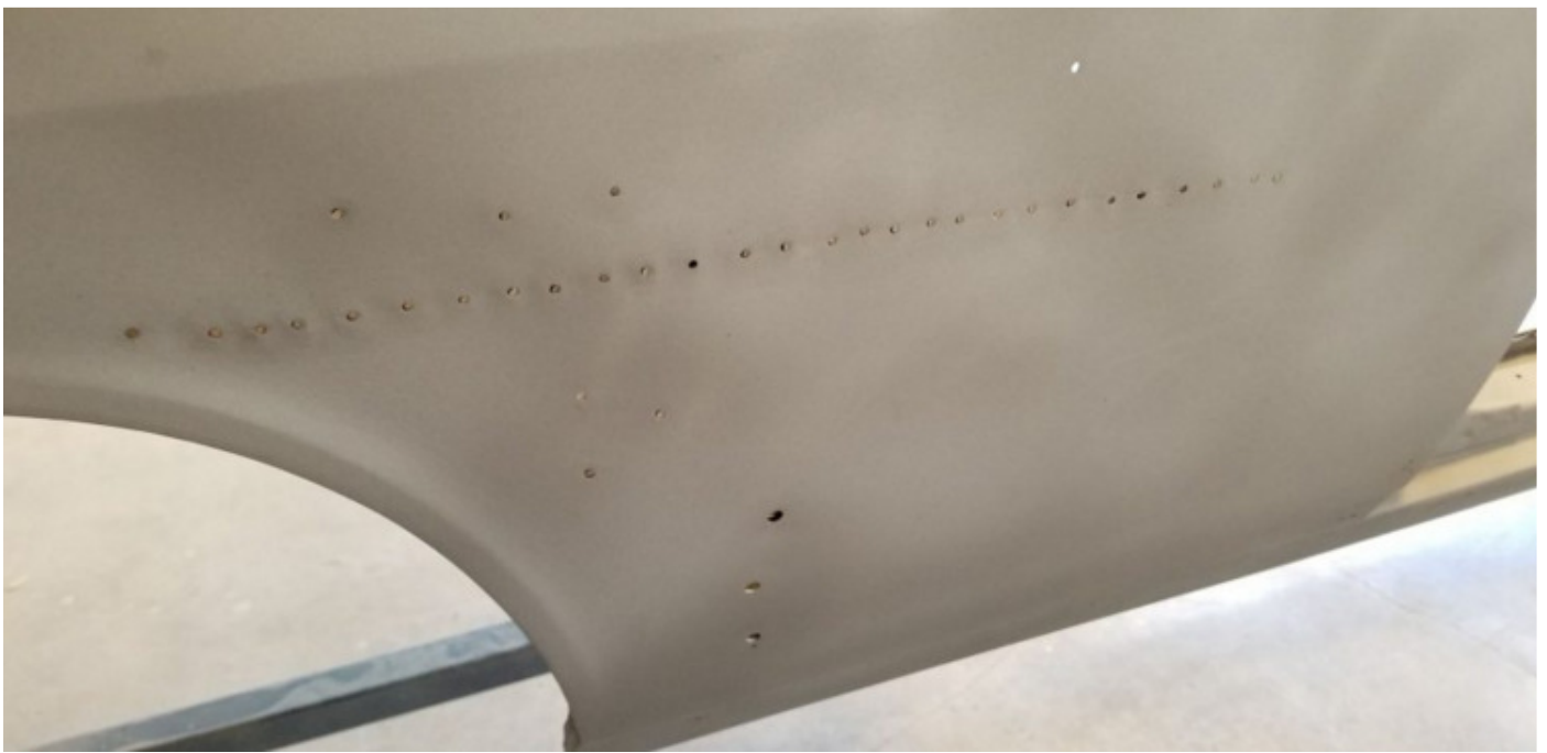
The left front fender which can still be saved.
