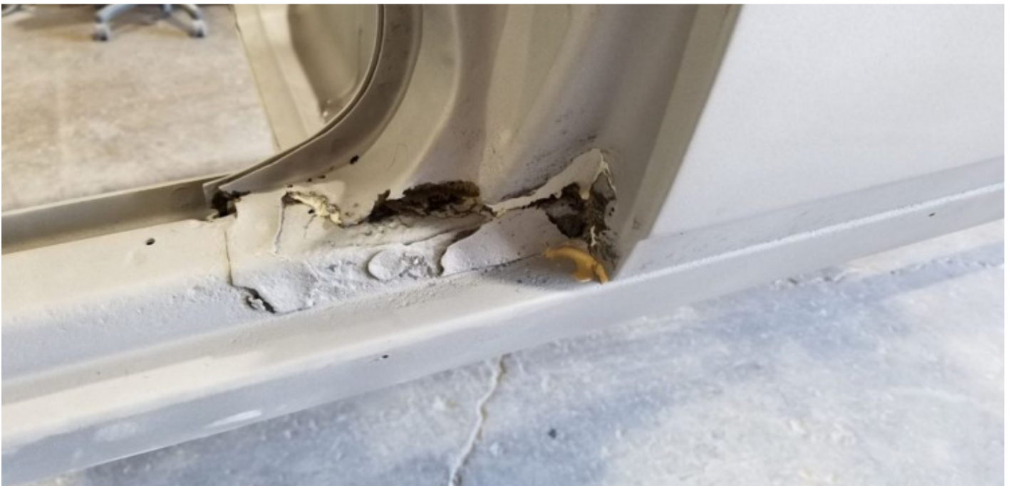
Corrosion at the rear of the driver's door sill. You guessed it – this was covered in Bondo as well.
