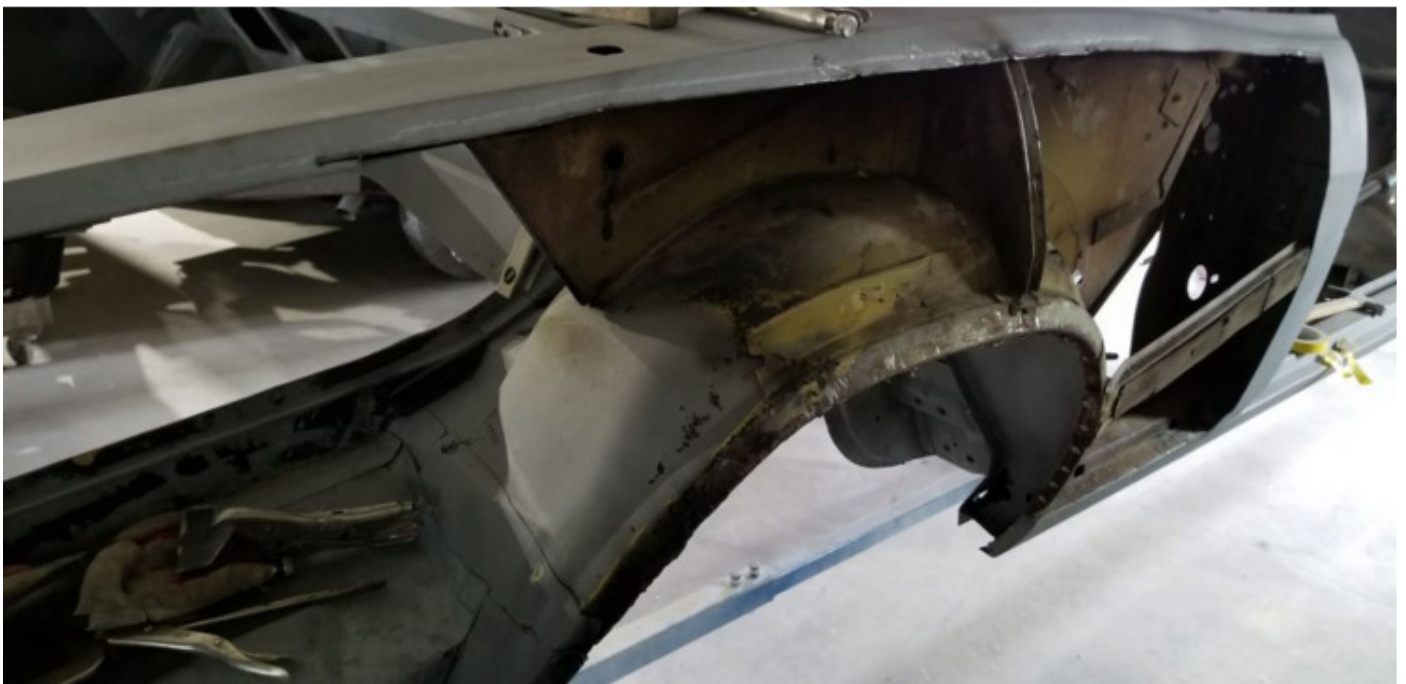
The right rear quarter panel has been cut off, awaiting a new old stock (NOS) replacement. The “repair” done by the former owner was too far gone to fix.
