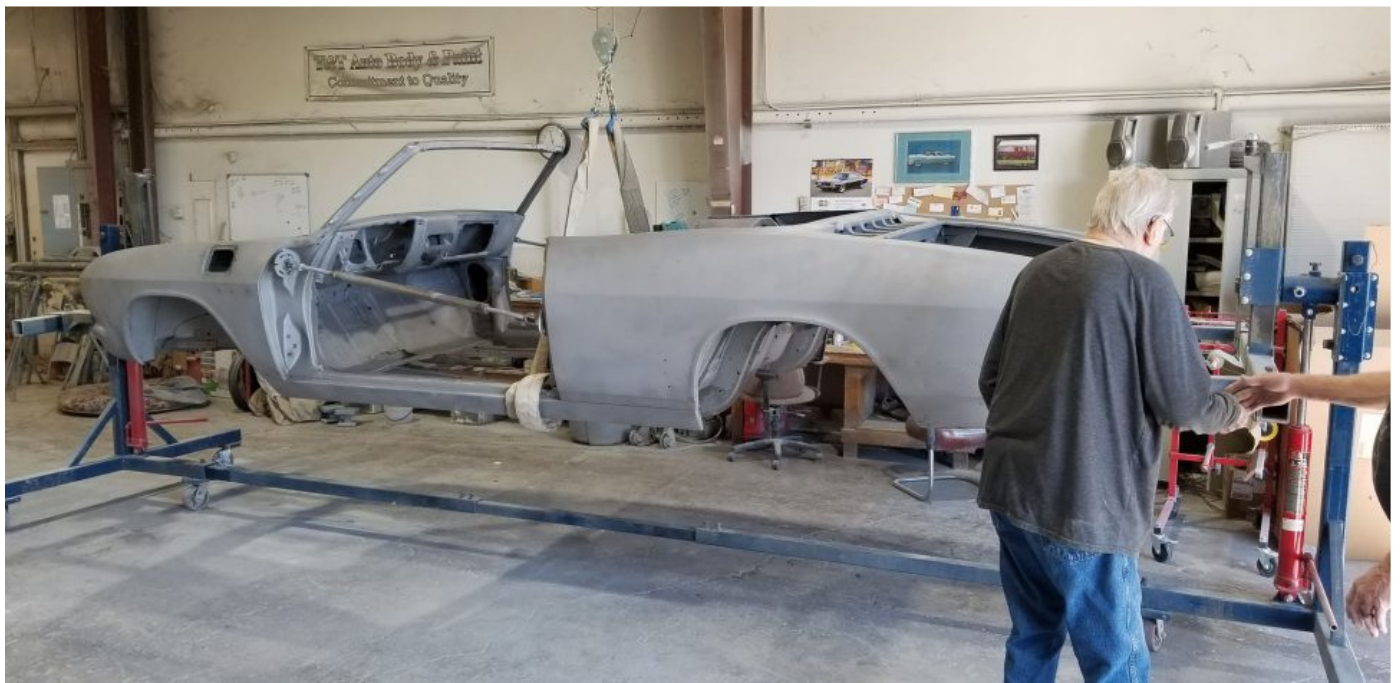
Installing the body shell — carefully — onto the rotisserie. Photos by author.
