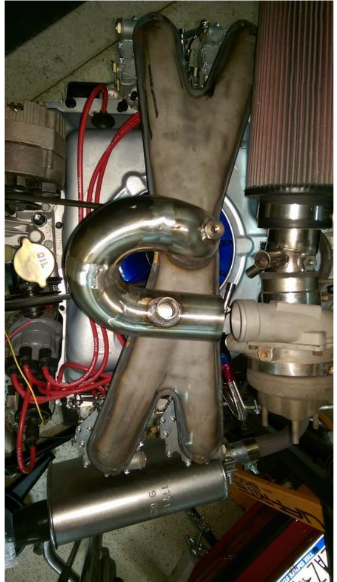
Welded ports for boost return valve, crankcase vapor return and methanol injection to air filter mount.
