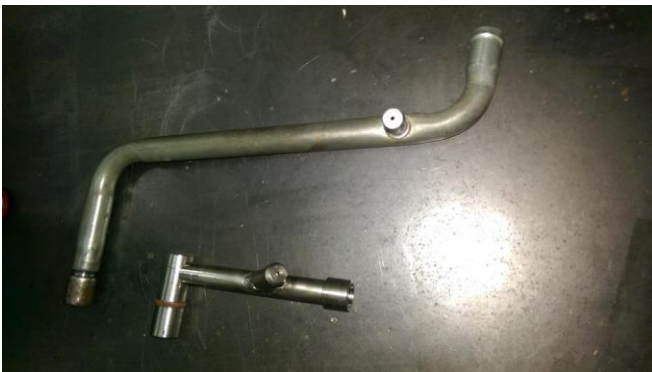
Tom made a custom fixed orifice pipe.
