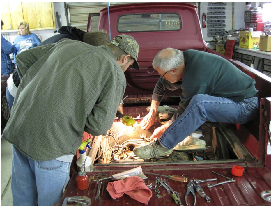
2009 Luna Tuna. Scott Allison "schools" his help on repair methods for the notorious manual choke Y used on 1961 Corvairs. Scott drove his LM sedan down from Kansas City, brought some treats, then spent his day helping others on their projects.
