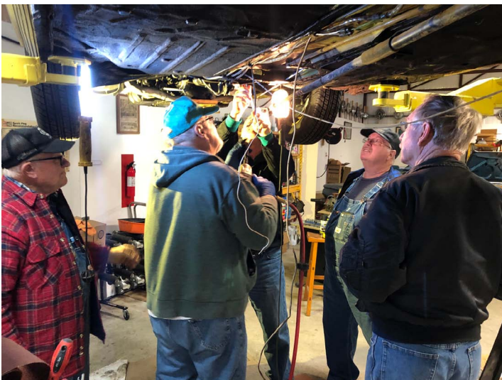
This Sunday mornings project was putting new transmission mounts into Ken's Spyder. Welte Photo.
