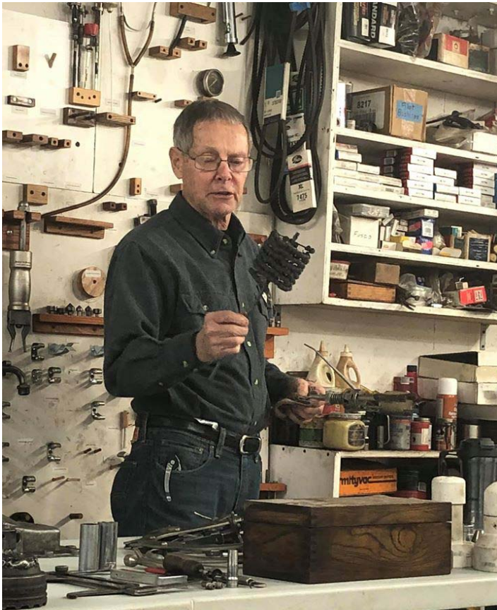
Mike explained the benefits of using a ball hone on Corvair engine cylinders. He also recommended the ball hone over the stone style for brake cylinders.
