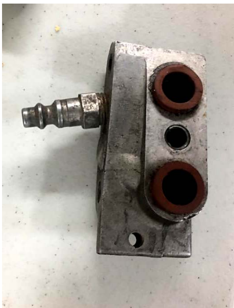
Many of the tools Mike displayed, he made. This oil cooler pressure tester was one of them. He also used PVC pipe sections and caps to create bearing and seal drivers. Bill Smith Photo.
