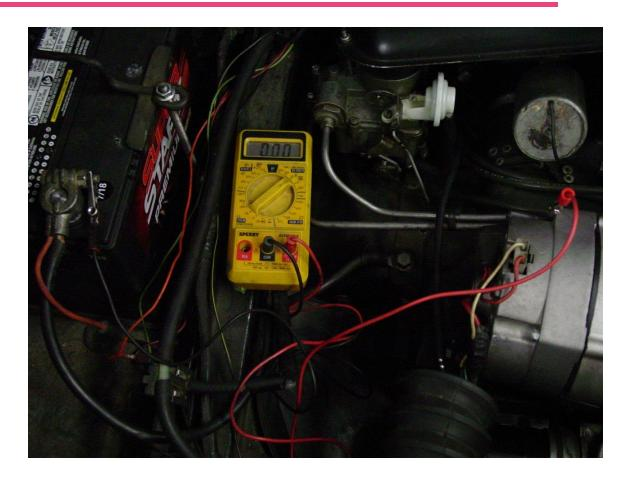
The voltage drop while cranking should be 0.20 volt or less.
