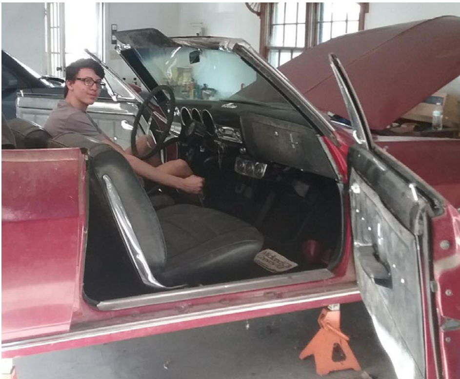
Devin tries out the driver's seat for size. Looks like a great fit. Lots of Glenn touches on the interior. A large tachometer clings to the steering column, with more gauges under the dash. Also a custom shifter.
