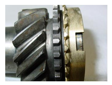
The above picture shows a new blocker ring with a 0.051 clearance.
