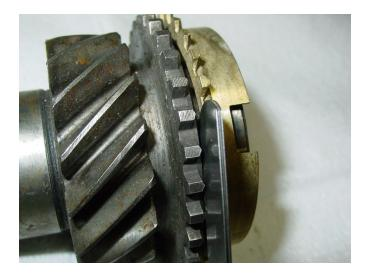
Use a feeler gauge to measure between the blocker ring and the spur gear ledge, holding the blocker ring against the gear while you measure. You need a minimum of 0.030 for used parts. New clearance is around 0.050.
