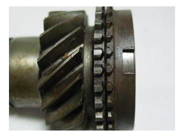
This picture shows a well worn blocker ring with a 0.025 clearance on the same gear.
