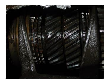
With the two shift forks in neutral, you can inspect second and third gear spur gear teeth and blocker ring clearance. Shift in to third and then into second and you inspect fourth and first gear teeth and blocker ring clearance alternately.
