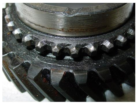
This picture shows spur gear teeth that have been flattened somewhat on their points due to worn out blocker rings and/or a driver missing hard shifts. This gear would work reasonable well if you used a new blocker ring but will continue to promote gear grinding with a badly worn blocker ring.
