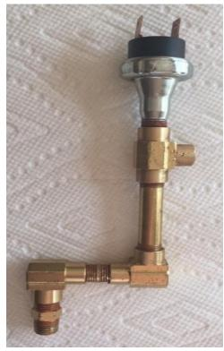
The oil light switch was moved to the Adaptabolt location. The pressure should have been nearly the same but apparently the oil pressure was lower at the bolt. I did not have a pressure gauge in order to measure the oil pressure, however. That did the trick. (Perhaps a very low-pressure oil pressure switch is available?)
