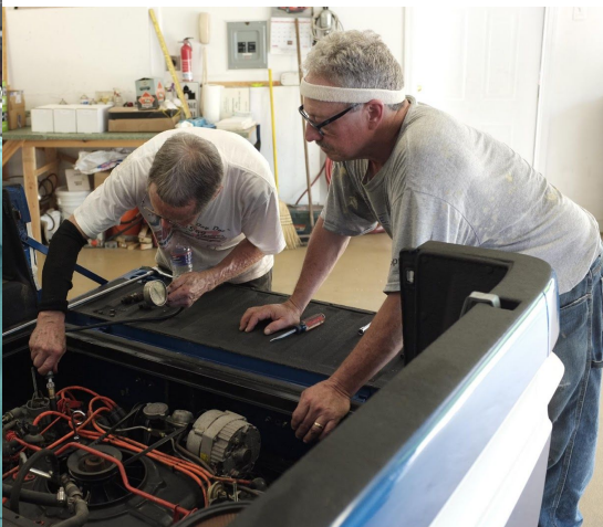
Above: Kevin Rafferty's Rampside getting a compression check; fortunately the miss was a valve spring and not a valve seat! Replacement was successful.
