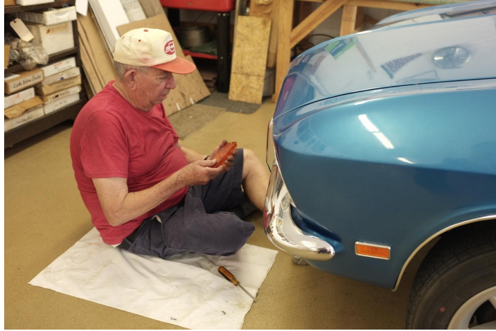
Above: Fred replacing a bulb in the front of his '69 before pulling sheet metal and checking an oil leak in the other end.
