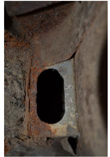
Looking Down into Opening into Rocker Panel, Visible When You Remove Interior Vent Covers
