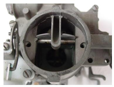
This top has a vent on either side of the inlet; some variations have a third vent hole in the "duckbill" and some have only a single vent hole in the "duckbill". All are susceptible to dirt from the air cleaner parts, gaskets and vents.
