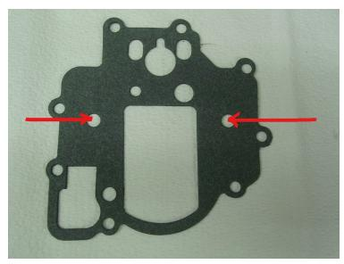
The two holes in the gasket on either side of the center opening are not far from the vent. Dirt can enter the float bowl as it rolls around on the gasket or gets washed into the bowl on a hard stop.
