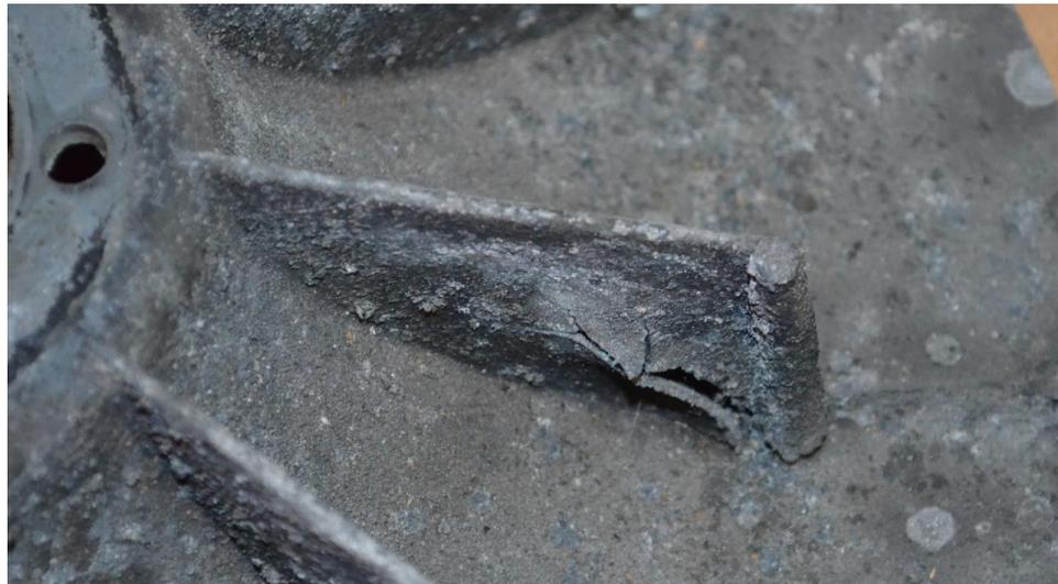
Late Model Magnesium Fan Corrosion
