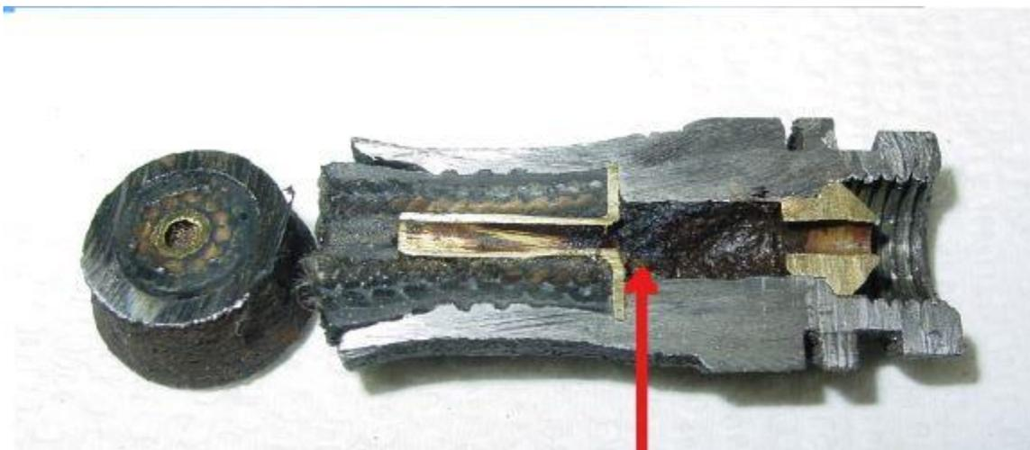
right side shows a longitudinal section of a brake hose with extensive clogging from corrosion.
