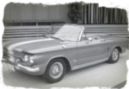
Corvair Sebring Roadster first version. It had a shortened wheelbase and was converted to a convertible from a coupe body.
