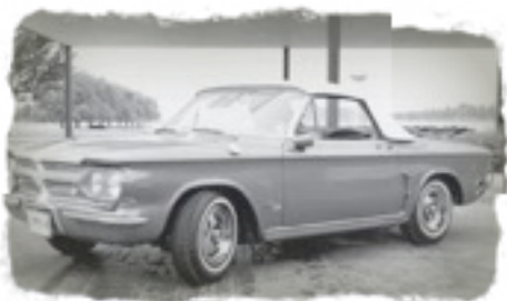
Sebring Roadster third version. The windshield and top from first version were reinstalled, as well as new one-off custom wheels designed by Styling. Bumperettes and rear fender exhaust outlets from second version were retained.
