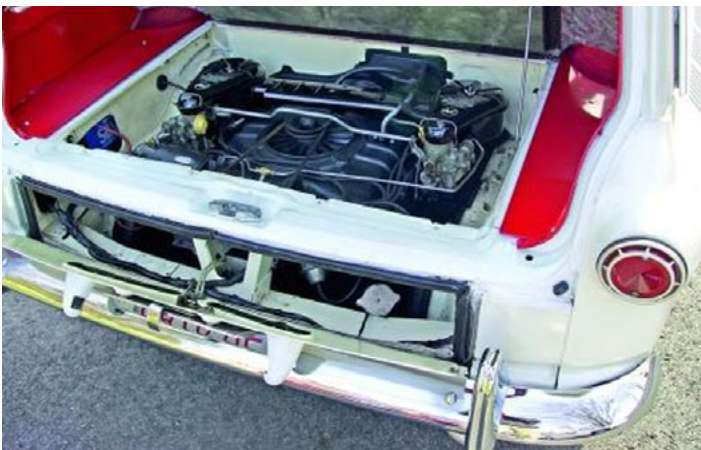
With the back of a Corvair station wagon loaded engine access is a narrow opening below the hatch.
