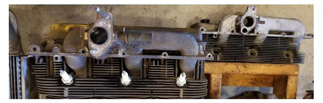
And this picture shows the boss where the pushrod tubes would have attached. Mike explained how one could change pushrod tube seals without removing the rocker arm bolts and therefore not losing torque of the head. You can see the two springs that I replaced.
