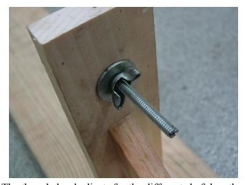
The threaded rod adjusts for the different shaft lengths.
