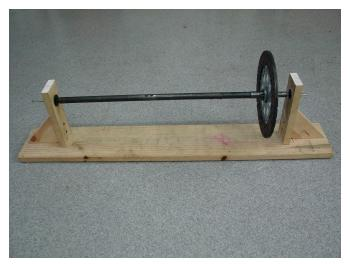
The above set up can check any clutch shaft and the disc.
