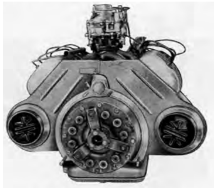
Above: This view shows the front of the engine with the ejector chambers removed. Note the star-shaped tail ends of the exhaust header pipes.
