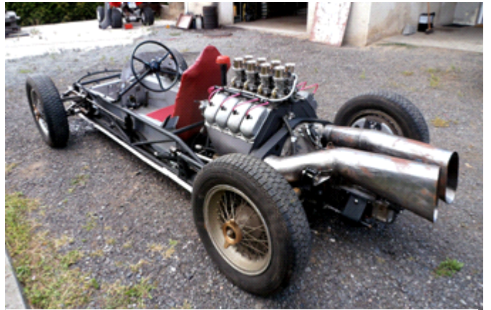
Tatra 607-2 chassis showing ejectors & diffusers
