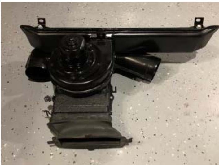
Heater blower motor all cleaned and repainted.
