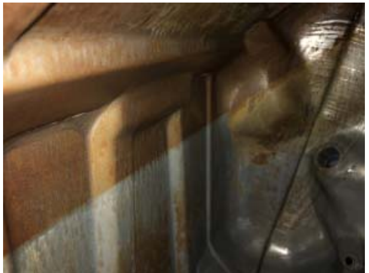
Gas tank in the process of being sealed with POR-15.
