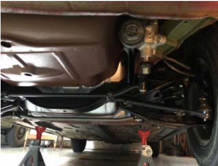
Front suspension with steering box completely installed. Sure looks nice.
