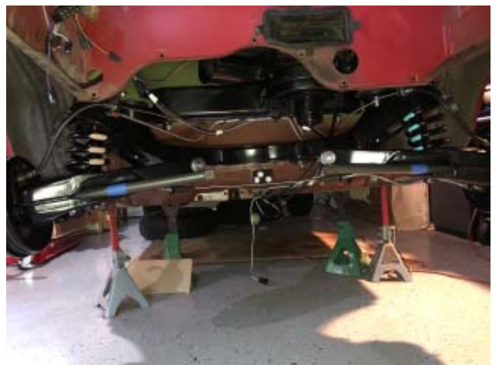
Rear suspension installed
