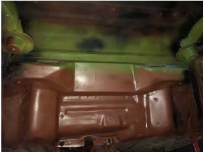
Underbody after green dichromate and red oxide primer.
