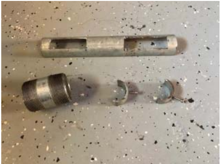
Some tools to help with pressing on/off the rear bushings.
