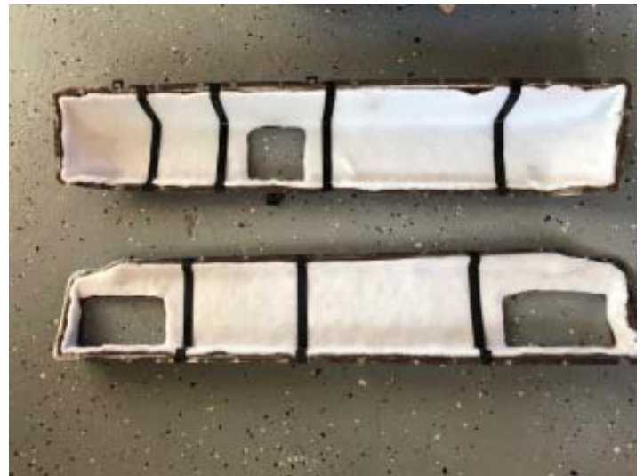
Heater box after being re-insulated. Good job!
