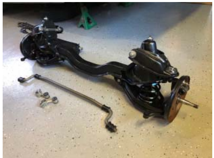
Front suspension after being cleaned, painted and rebuilt. What a transformation. Looks brand new!
