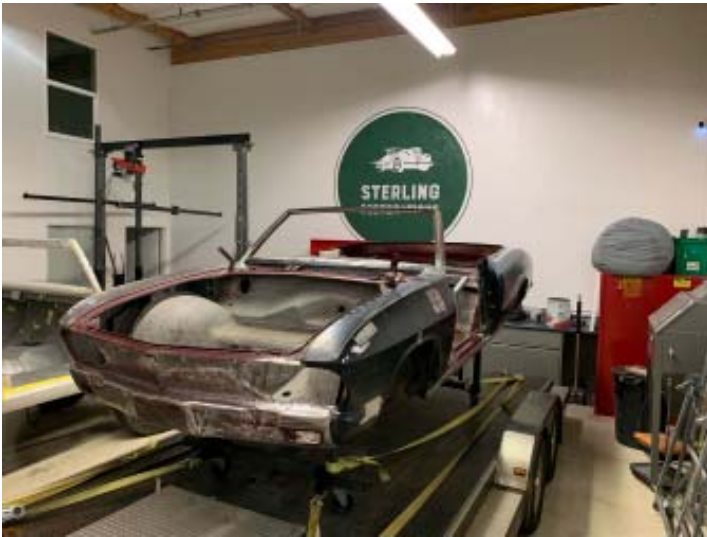
A couple of pictures taken after the new front and rear fenders have been welded in place.
