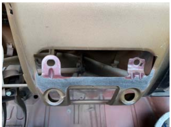
Someone had removed the stock radio mounting ears to install an after-market radio. Bruce somehow found the missing parts and had them welded back in place. When painted you won't be able to tell anything was done!
