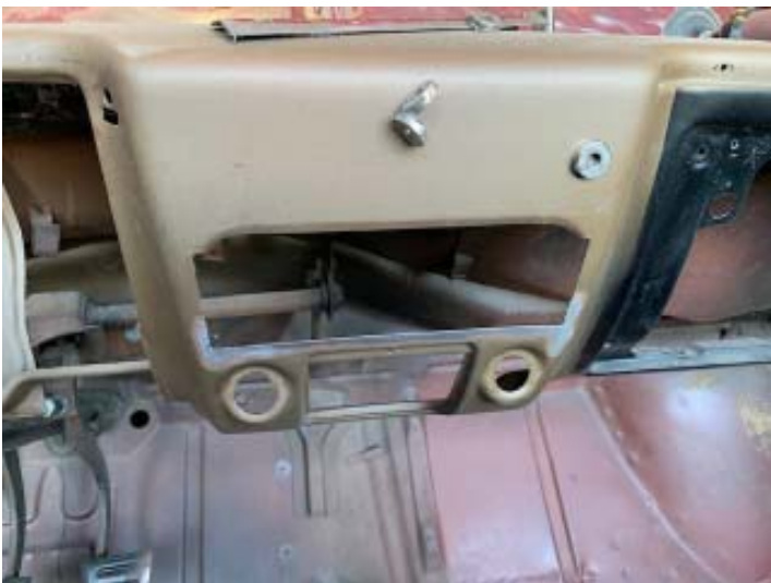
Someone had removed the stock radio mounting ears to install an after-market radio. Bruce somehow found the missing parts and had them welded back in place. When painted you won't be able to tell anything was done!
