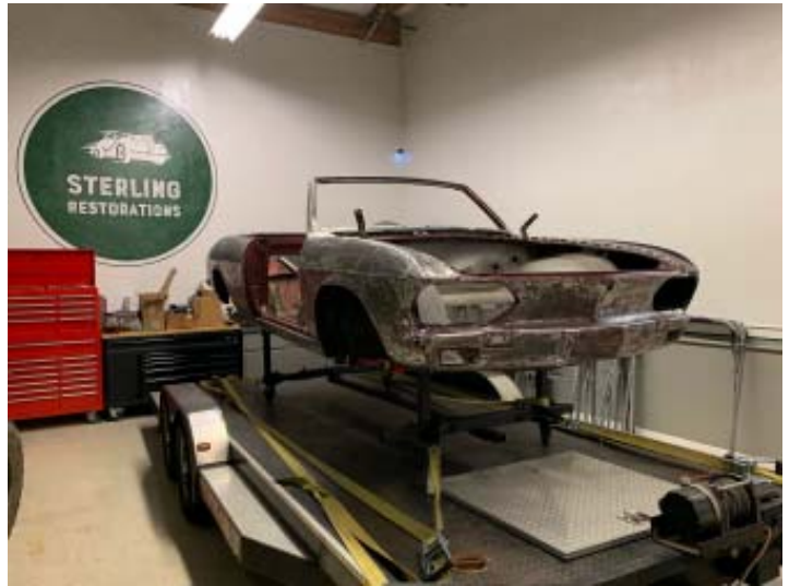
A couple of pictures taken after the new front and rear fenders have been welded in place.
