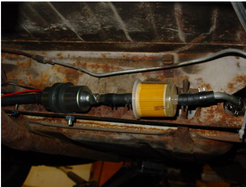
Greenbrier Fuel Pump Installation
