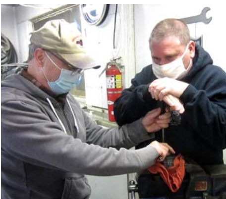
ABOVE: Mark Welte (left) and Keith Hammett ground on an old screwdriver until it became the perfect tool to remove stubborn Corvair carburetor jets.
