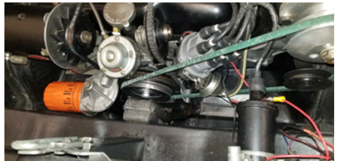
This is the completed set up. The red hose in the back is the chimney tube taking heat directly from the exhaust manifold to the choke thermostat. This Holley carburetor was used originally on '57 Ford small V8 trucks. The air cleaner was a pain to locate. I wanted a bigger air cleaner which was not typical for a smaller intake like this one or a Corvair.
