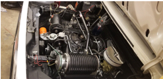
This is the completed set up. The red hose in the back is the chimney tube taking heat directly from the exhaust manifold to the choke thermostat. This Holley carburetor was used originally on '57 Ford small V8 trucks. The air cleaner was a pain to locate. I wanted a bigger air cleaner which was not typical for a smaller intake like this one or a Corvair.
