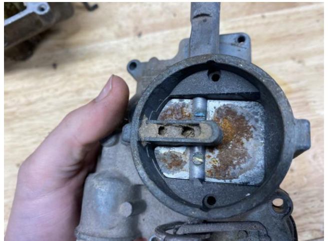
Here is the choke plate in the closed position, where it serves to restrict air from entering the engine, causing a richer air/fuel mixture. Photo by Kyle Smith | Hagerty Media Site
