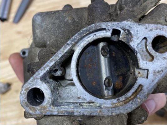
The throttle plate in the closed position. Photo by Kyle Smith | Hagerty Media Site
