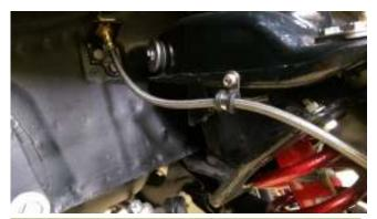
Made one more addition, because I did not move where the stock hardline was located the flexible line passes behind the spindle. Wanted to make sure that if I hit a large bump that the bumper would not pinch the line. It might not have anyway, but I did this: (has slip fit so it can move in and out some)
