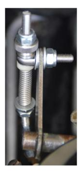
Basically, the lower clip is used but instead of using a threaded swivel and clip at the top, a smooth bore rod end is used that slides up and down as you adjust. To allow the movements yet hold position once adjusted, a compression spring is used to restrain the rod end. To make it "deluxe", you can even use a knurled adjusting nut (as shown in the photo). To allow movement at the pivot points, washers are used and are adjusted to not bind.
