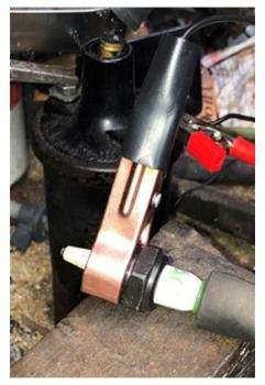
That's when I noticed the ground clip on my special sparkplug (shiny copper thing in the photo), the plug with the EXTENDED tip was sitting on the vise where I had placed it before I clamped the Distr in that same vise to hold it, while I tested it...(!)
