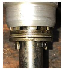
After adding the new washer, the shaft no longer wiggled up/down in the Distr, and still spun easily, so I felt I had done my duty and put the Distr on the bench. It went right next to the coil that I use to test fire such things as Distrs that I have just fiddled with, so I thought - why not make certain this guy's functioning...properly.
