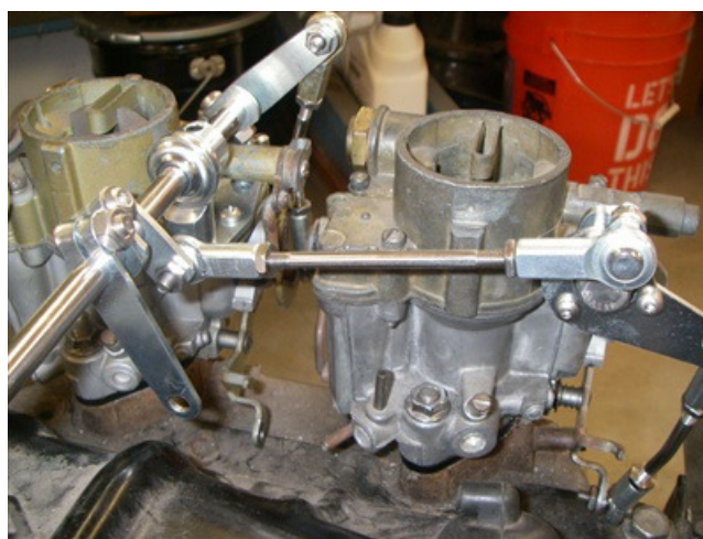
NEW – 140hp Non-Progressive Linkage. All 4 Carbs move as one - Left Side Shown. Appearance is just like the 1965 140hp Linkage. Will work on 1966-69 140hp with the Choke Lock-outs removed.
