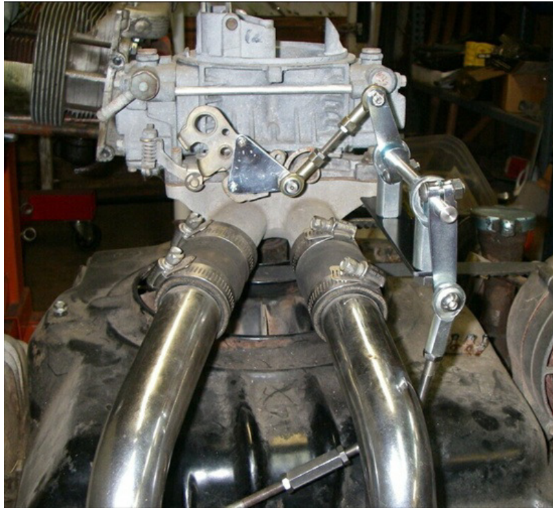
Holly 390 4 Barrel Linkage. You do not need to modify your stock Accelerator Rod to install this kit.
