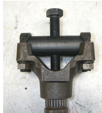
Yoke Puller installed for use On 1960-64 Axle
