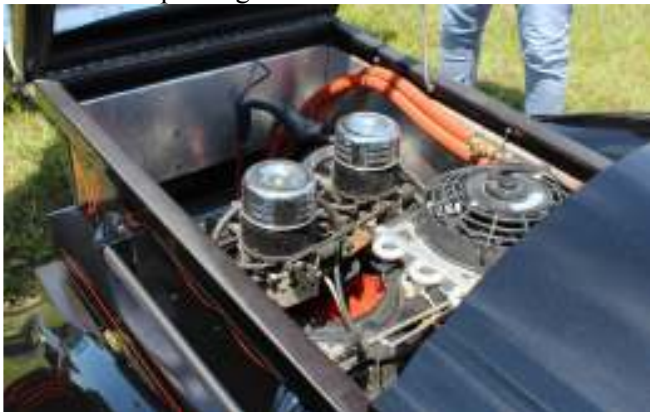
Those are 2 throttle bodies for fuel injection on the Corvair motor. Mounted inboard.
