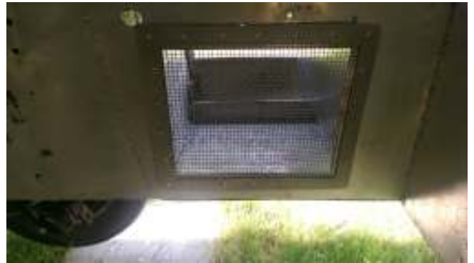
Made a bit more forward progress. Installed a intake path for fresh air, like the later coaches. Added a door inside to separate storage in rear, still have to add latch and finish outer door grill. Also put the engine/Trans back in. Tom Koprevich
