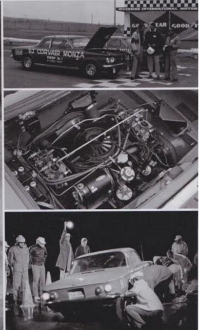
tachometer, Empi front sway bar, Shelby-branded steering wheel, dual Moon fuel tanks (to aid in accurately measuring fuel economy), Goodyear Blue Streak tires, and Lucas driving lights. The second car got those parts too, but was also fitted with Thomas' fourcarb induction setup, a Racer Brown camshaft, Hands magnesium racing wheels, sintered metal brake linings, and open exhaust. They're easy to tell apart in the photos by their numbers: 985 for stock, 98M for modified.
