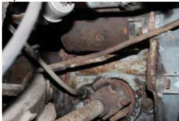
Removing the wheel is the best way to access the starter on an early
