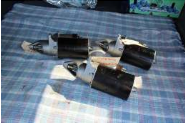
Three starters all rebuilt and like new. Tags attached with date of manufacture.
