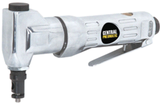
An example of a pneumatic nibbler.
