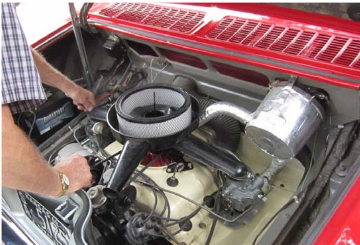
Roy Juenemann has been experimenting with ways to reduce the hot start cranking on his LM Corvair. In his latest version he installed heat shields and a fan.
