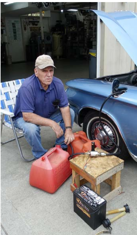
Chuck Morris waits patiently as he drains gas from his EM convertible. Next step was to replace a bad float on the fuel sender.
