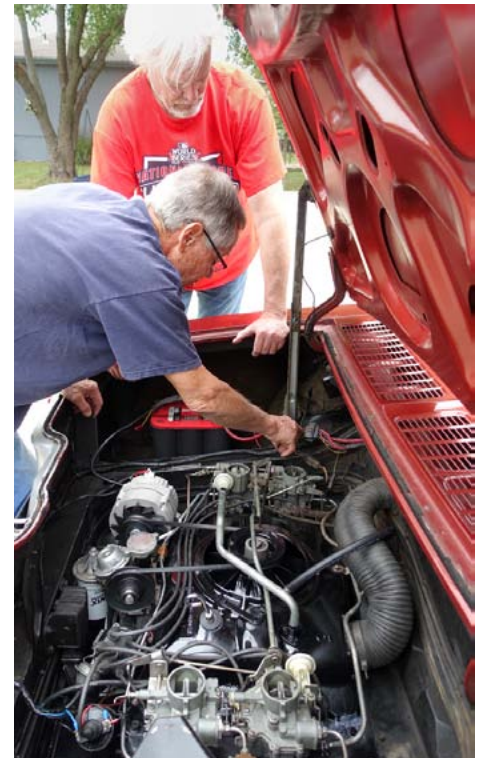
ABOVE: Mike Dawson balanced and adjusted the carbs on Don D's 140 Aztec Bronze Corsa.
