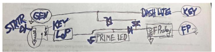
HA! The '66 has the Special engine, (180 psi on cranking) which required a BIGger starter motor, [Clark's Gear Reduction Starter Motor] which doesn't come with a yellow wire (the resistor bypass) so when the KEY input got latched over to the NO contact it Latched the Relay but also sent a signal back up that wire and kept the Starter Motor engaged! So, a diode had to be added into that control circuit. You can see in the drawings, above, they went back into the sketches, and added that diode.
