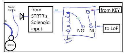
The wire from the STARTER Relay (the Original big Purple wire) is tapped at its original connector, near the Umbilical. Note lack of the Yellow wire. This tap provides the control signal for the Latching Relay.
