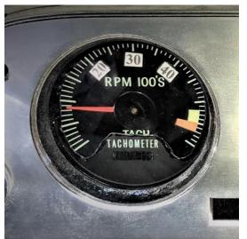
Turns out the guts of the two units would fit inside either can. The Late Model just sits inside a bigger box. BUT, it has a  $270^{\circ}$  movement so it will give me a nicer swing to the needle, I think. A close-up shows my butchering, next time I will paint better.
