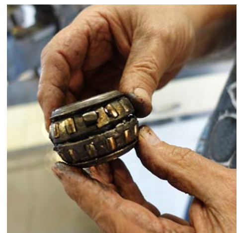
Dennis' bad bearing. One of the rollers had turned sideways.
