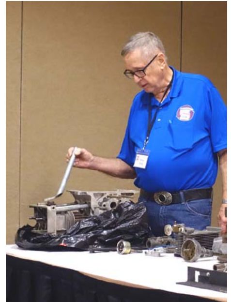
ABOVE: Elvis King presented a Tech Talk on Friday afternoon. He explained some of his homemade Corvair tools. Here he demonstrates a push rod tube remover.
