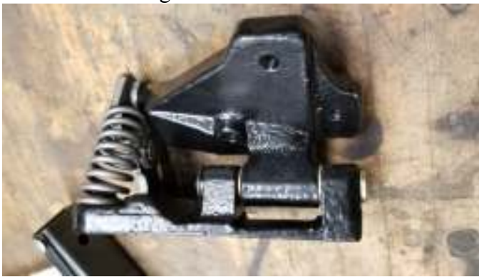
Rebuilt and powder coated door hinges including new brass bushings.
