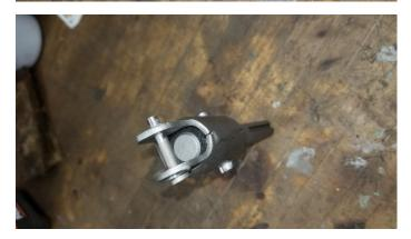
Added hardened roll pins in the holes tig tacked them in place, reamed out openings. (Should prevent wear over time) Made a 95 durometer bushing out of TPU, noticably stiffer than what was left of stock but not super hard like nylon.
