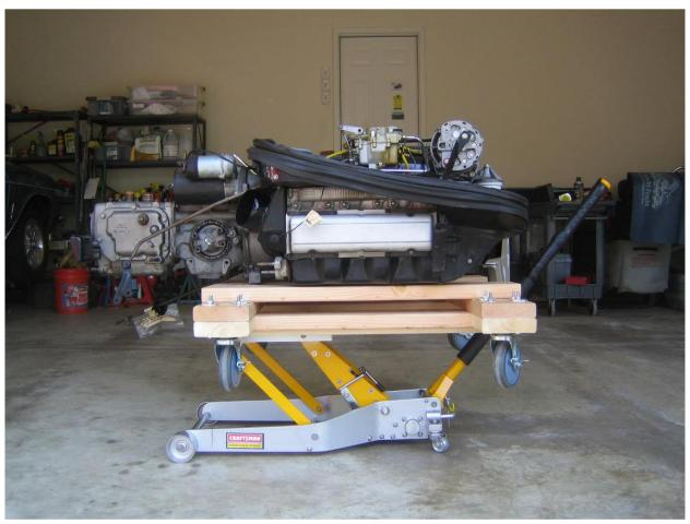
add an extra inch wood pad between the caster wheels and the rest of the cradle to get the clearance needed for the ATV jack.
