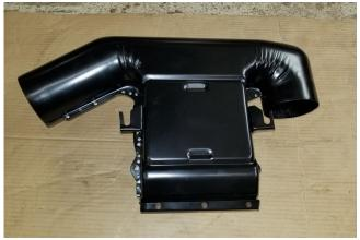
Finely used some stainless rivets to assemble the halves and modified the "air" inlet and blocked it off since I will not be using it.
