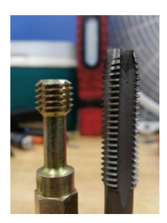
When Joe went to replace the pilot bearing he tried the "wet bread" technique he saw in Dave Motorhead's video. Didn't work for him. He they tried very thick grease and this did work. Tim said you can just use a 5/8" bolt. Thread it in until it bottoms out and then keep running and the bearing come out. You may have to toss the bolt afterwards.
