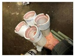
2" PVC plumbing pipe with a straight coupler. This allows me to slip the coupler onto the carb with the pipe coming into it. Had to cut and paste a bit to make it fit nicely, where I wanted it, but a little BONDO is a wonderful thing. There are bumps on the carb that
