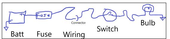
wire all the way through the switch to the Load (a Motor or the Glove Box Light) and eventually to ground. That's what a circuit was like in the old days.
