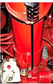
To hold these tall guys down on top of the carbs I had to make looonger "Fran Schmit Spring Loaded J-hooks" - 6 inches long! Turns out I had a nice piece of iron wire that bent when heated and otherwise lent itself to fabrication. With the stacks and the 'Big-X" air cleaner mounted, I can grab the cleaner and shake the car and nothing moves. I think I'm ready to run a test at 6000+RPM and see if they allow the air to turn that corner - smartly! Stay tuned!
