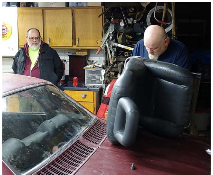
Owen Strawn looks on as Bill Smith works on the first project of the day. Bill was transferring the seat tracks from the old seats to his new ones.
