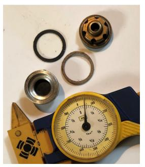
The thing that I didn't expect, was the existence of a teeny little gasket underneath the check valve — where it seats into the housing. This would, I presume, reduce any leakage around the closed valve when it is holding back some pressure. It's only
