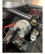
stock radio utilizes a 3-amp fuse. With the upgrades it now requires a 10-amp fuse in the stock fuse block under the dash. All components are feed from the stock battery location with an inline 125-amp fuse.
