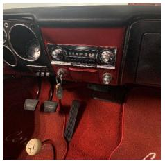
5. In all this install required drilling 12 holes for either wiring or bolt mounts. No holes were cut for the speakers and the radio utilizes the stock radio and mounting brackets. The largest hole is 1" in size and is located on the trunk/passenger wall. This location is where all speaker wiring is located. Primary power was routed from the engine compartment along the left under the seal plate to the trunk. These were both 1/2" holes. All large holes can be
