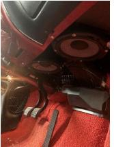
it without drilling holes in the floorboard. Second, while it fit under the seat nicely, no one would be able to sit in the seat as they would be resting directly on the speaker and eventually would cave the speaker grill in with use, another solution was required. Mounting the unit inside the rear seat back rest was proposed. Utilizing two metal supports, proceeded to drill four small bolt holes to mount to the seat frame. Speaker/amp is mounted so that it faces forward in the car to
