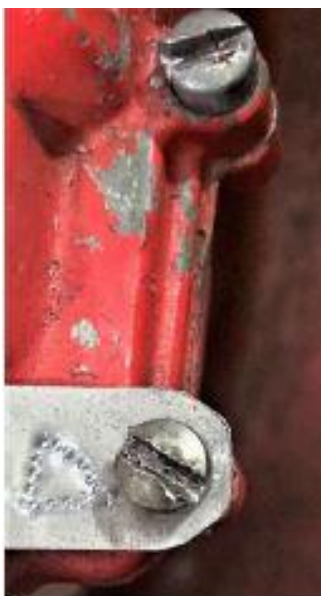
Bunged up (that's a technical term) Slotted Screws
