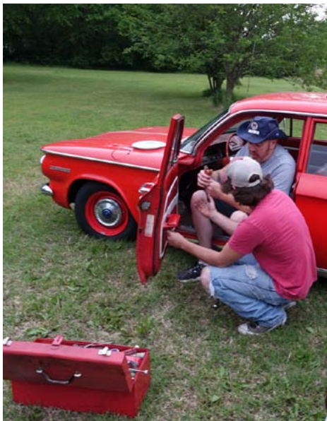
Jason and Nick Pool had a quick fix-it session for a window regulator that went off track.
